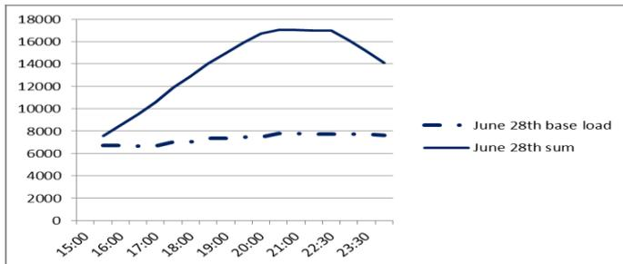
Fig. 4 The graph shows a scenario for June 28<sup>th</sup> where 100% of the inbound traffic to Hvaler requires recharging. The aggregated effect caused by the 3,3kW chargers have been superimposed on the base load for that day. X-axis shows the hour of the day. Y-axis shows the accumulated effect in kW.
