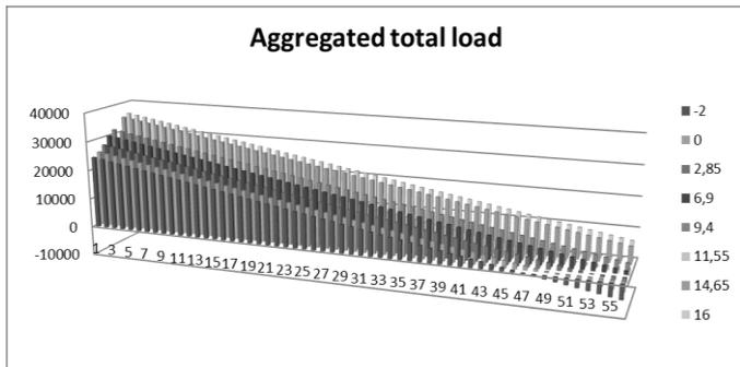
Fig. 10 The combined loads  $L_{PEV}$  and  $L_{base}$  plotted against the day temperature (x-axis) and Month Mean Temperature (the horizontal axis orthogonal to the X-axis). The likelihood of the temperature combinations will differ according to local weather statistics.
