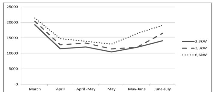
Fig. 13 Aggregated load curves based on actual records for max base load in the net and observed traffic intensity plotted against calendar period. Notice the distinct U-form obtained.
