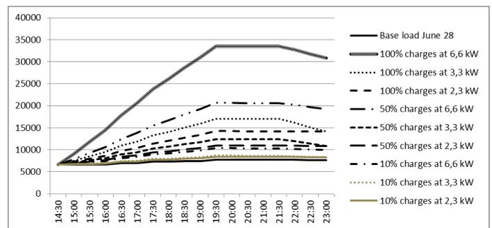
Fig.6 Different charging scenarios plotted for June 28<sup>th</sup>, 2013. X-axis shows the hour of the day. Y-axis shows the accumulated effect in kW. The base load increases slightly during the evening and reaches approximately 7,7MW
