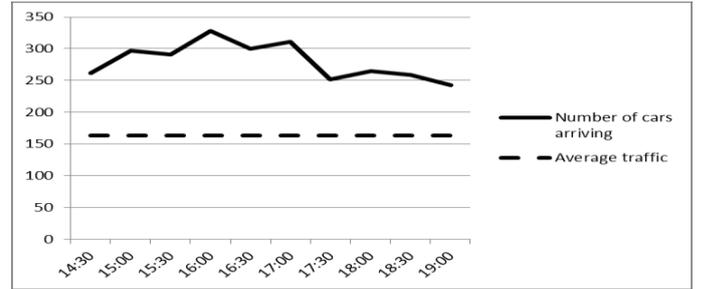
Fig. 2 The traffic intensity for Hvaler plotted against time on June 28<sup>th</sup>, 2013. X-axis shows the hour of the day. Y-axis shows the number of cars per 30 minutes.
