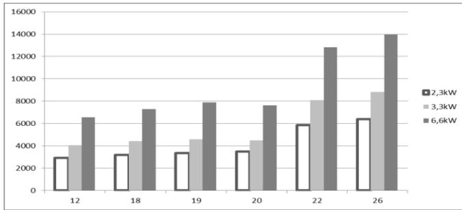
Fig 8 The graph shows the average load  $L_{pegv}$  in kW (y-axis) for peak hours, plotted against calendar time (week number).
