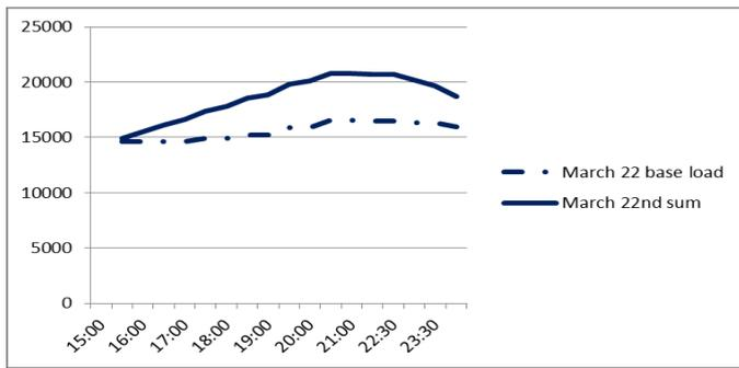
Fig.3 The graph shows a scenario for March 22<sup>nd</sup> where 100% of the inbound traffic to Hvaler requires recharging. The aggregated effect caused by the 3,3kW chargers have been superimposed on the base load for that day. X-axis shows the hour of the day. Y-axis shows the accumulated effect in kW. A similar scenario is shown for June 28 in Fig. 4. The relative importance of charging is clearly shown.
