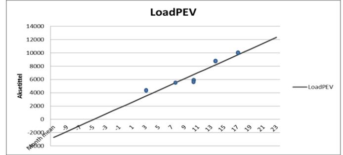
Fig. 9 Linear regression based on the observations shows the relationship between the mean temperature for a given month and the load potentially imposed on the grid based on a scenario where 100% of the vehicles will start to recharge at time of arrival.
