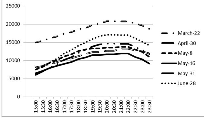
Fig. 7 The graph shows a 3,3kW scenario for different dates during spring 2013. Each line represents a situation where all traffic at the dates shown requires recharging of batteries. The accumulated load has been superimposed on the base load for that day. X-axis shows time of day. Y-axis shows effect in kW.
