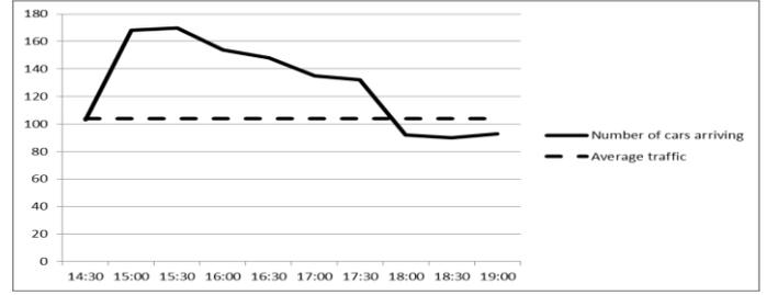
Fig. 1 The traffic intensity for Hvaler plotted against time on March 22<sup>nd</sup>, 2013. X-axis shows the hour of the day. Y-axis shows the number cars.
