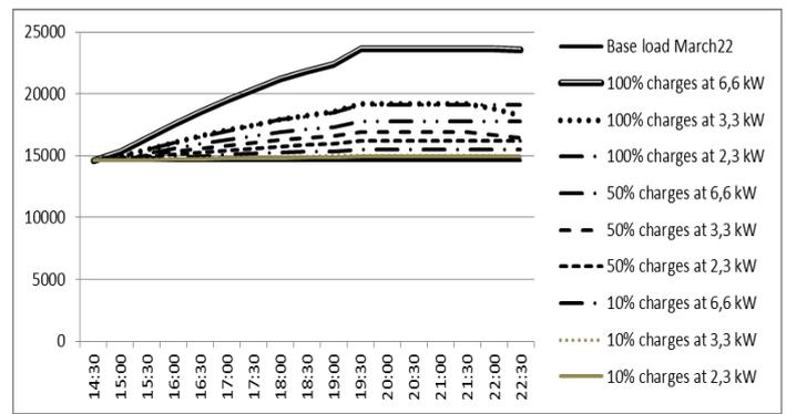
Fig. 5 Different charging scenarios plotted for March 22<sup>nd</sup>, 2013. X-axis shows the hour of the day. Y-axis shows the accumulated effect in kW. Notice that the base load is varying slightly around 15MW.
