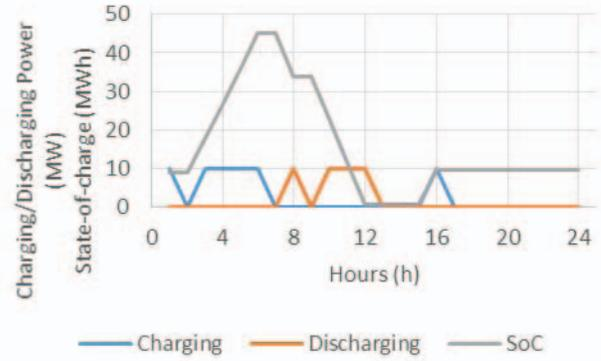
Figure 4. BES operation: charging, discharging, and SoC during the day
