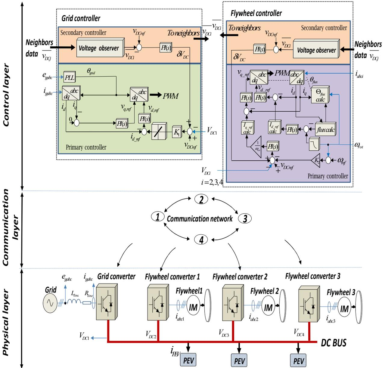
Fig. 2. Flywheel and grid converter control schemes
