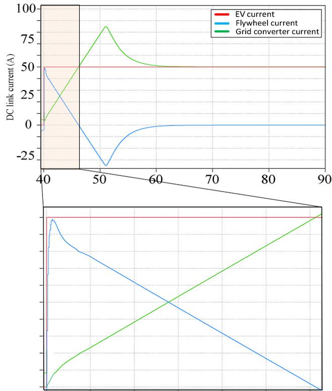
Fig. 6 DC link current of PEV, GC and FC
