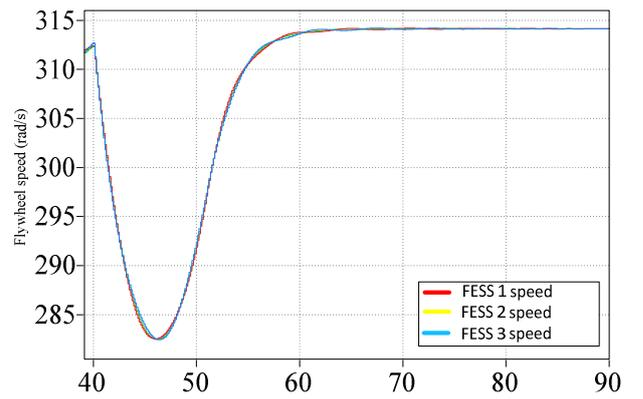
Fig. 5 paralleled FESS rotational speed
